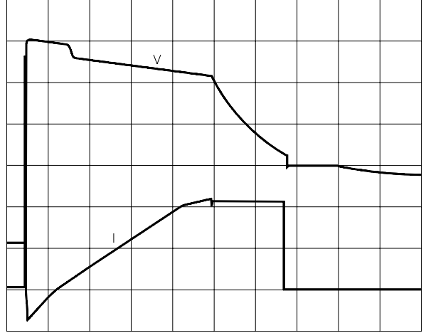
Figure 21 : Voltage Drop on the Yoke and Current Flowing through the Boucherot Cell - V = 10V/div. I = 100mA/div. - t = 100\mu s/div.
