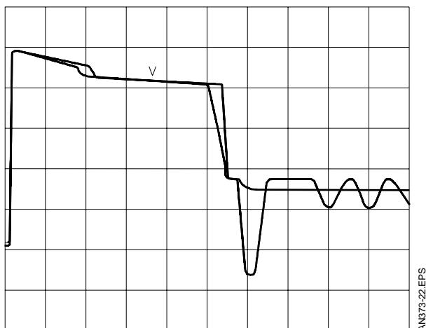
Figure 22 : Effect of Resistor in Parallel connected to the Yoke V = 10V/div.
