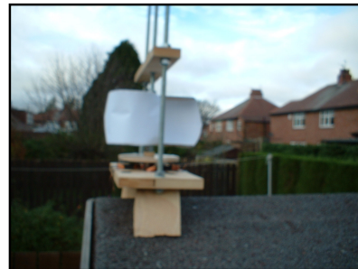
Figure 2: the model turbine (end view)
